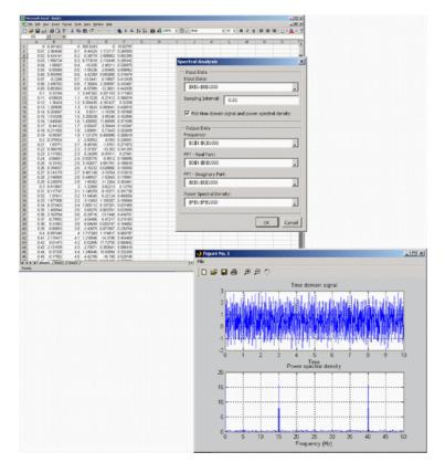
The power spectral density reveals the two signals at 15 Hz and 40 Hz.
